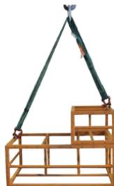
If the lifting points are an equal distance on either side of the center of gravity but one is higher, the double leg should be attached to the higher lifting point
