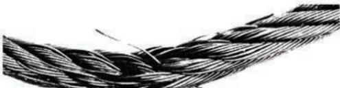
**Reverse bending.** Running this rope over one sheave and under another caused fatigue breaks in wires.
