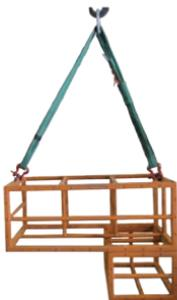
If one of the lifting points is closer to the center of gravity, attach the double leg to this lifting point. It will have the highest weight concentration. If the Twin-Path® Adjustable Bridle is attached so that the single leg is nearest the center of gravity, the lift cannot be made.
