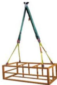
The Twin-Path® Adjustable Bridle should be used in applications where the double leg horizontal angle is greater than 45 degrees. Always connect above the center of gravity. If connections are made below the center of gravity, the load may turn when moved.
