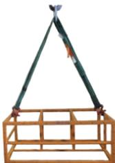
If the lifting points are equal distance from the center of gravity, the Twin-Path® Adjustable Bridle can be hooked up with the double or single leg on either lifting point
