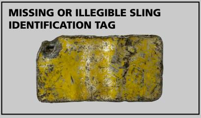
IF YOU IDENTIFY ANY OF THESE TYPES OF DAMAGE IN A SLING, REMOVE IT FROM SERVICE IMMEDIATELY EVEN IF THE DAMAGE YOU FEEL OR SEE IS NOT AS EXTENSIVE AS SHOWN IN THE PICTURES. SLINGS THAT ARE REMOVED FROM SERVICE MUST BE DESTROYED AND RENDERED COMPLETELY UNUSABLE UNLESS THEY CAN BE REPAIRED AND PROOF-TESTED BY THE SLING'S MANUFACTURER OR OTHER QUALIFIED PERSON. YOU MUST NEVER IGNORE SLING DAMAGE OR ATTEMPT TO PERFORM TEMPORARY FIELD REPAIRS OF DAMAGED SLINGS
