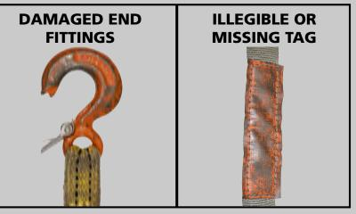
IF YOU IDENTIFY ANY OF THESE TYPES OF DAMAGE IN A SLING, REMOVE IT FROM SERVICE IMMEDIATELY EVEN IF THE DAMAGE YOU FEEL OR SEE IS NOT AS EXTENSIVE AS SHOWN IN THE PICTURES. SLINGS THAT ARE REMOVED FROM SERVICE MUST BE DESTROYED AND RENDERED COMPLETELY UNUSABLE UNLESS THEY CAN BE REPAIRED AND PROOF-TESTED BY THE SLING'S MANUFACTURER OR OTHER QUALIFIED PERSON. YOU MUST NEVER IGNORE SLING DAMAGE OR ATTEMPT TO PERFORM TEMPORARY FIELD REPAIRS OF DAMAGED SLINGS
