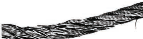
Undersize sheave grooves. Sheaves were too small, causing strands to pinch. Wires then fail in the valley between the strands.
