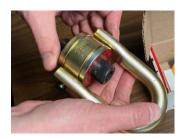
Locate hoist ring assembly and visually inspect for any issues.
