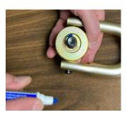
After the inspection, the hoist rings should have an identifier added, that indicates the inspection was performed and found to be acceptable. In this case we placed a blue paint pin dot next to the E-Clip.
