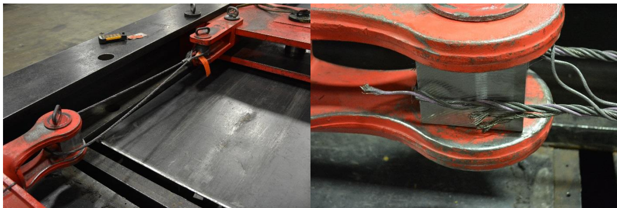
Figure 3 – Wire Rope Cut Test
