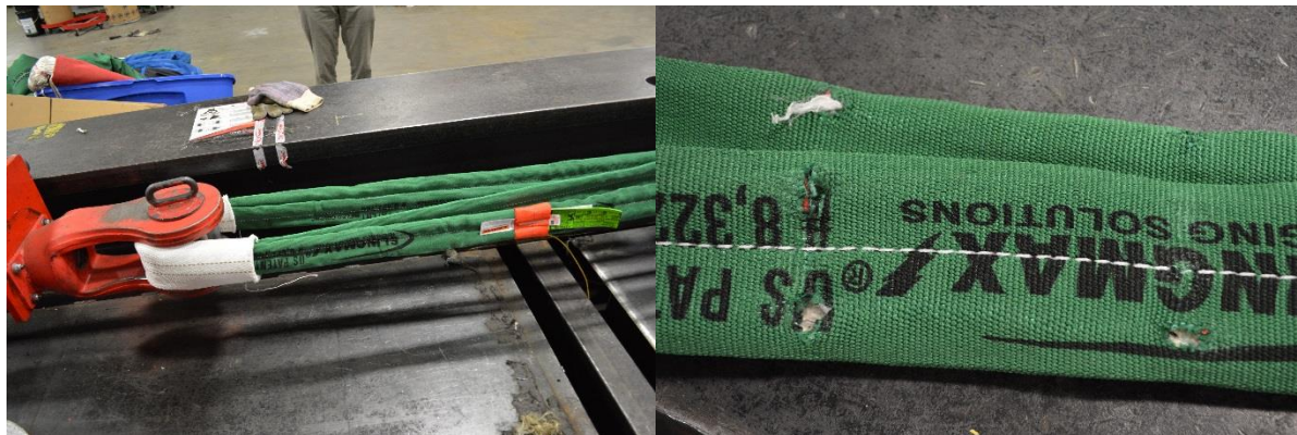
Figure 7 – Wire Rope Sling with Cornermax Sleeve Cut Test
