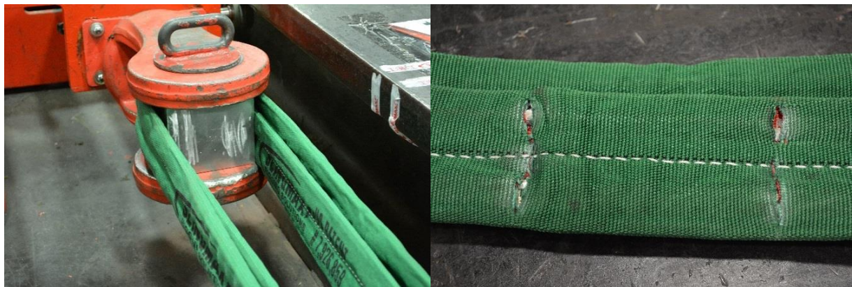
Figure 5 – Polyester Roundsling Cut Test
