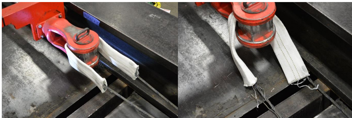
Figure 7 – Wire Rope Sling with Cornermax Sleeve Cut Test
