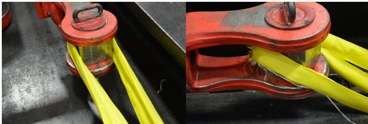
Figure 5 – Polyester Roundsling Cut Test
