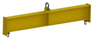
For lifts where height is severely restricted, Modulift can design and manufacture Low-Height Lifting Frames. Similar to Spreader Frames, but whereas Spreader Frames have top Slings attached between the frame corners up to the crane hook in the centre, instead a Lifting Frame generally has no top slings – rather the crane hook attaches directly to a large lug on the top of the frame in the centre
